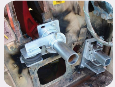
Skalper MDX and Razorback MDX with dual Air-Shoc tensioners installed on this 48" conveyor system handling 4000 tph of copper ore.
